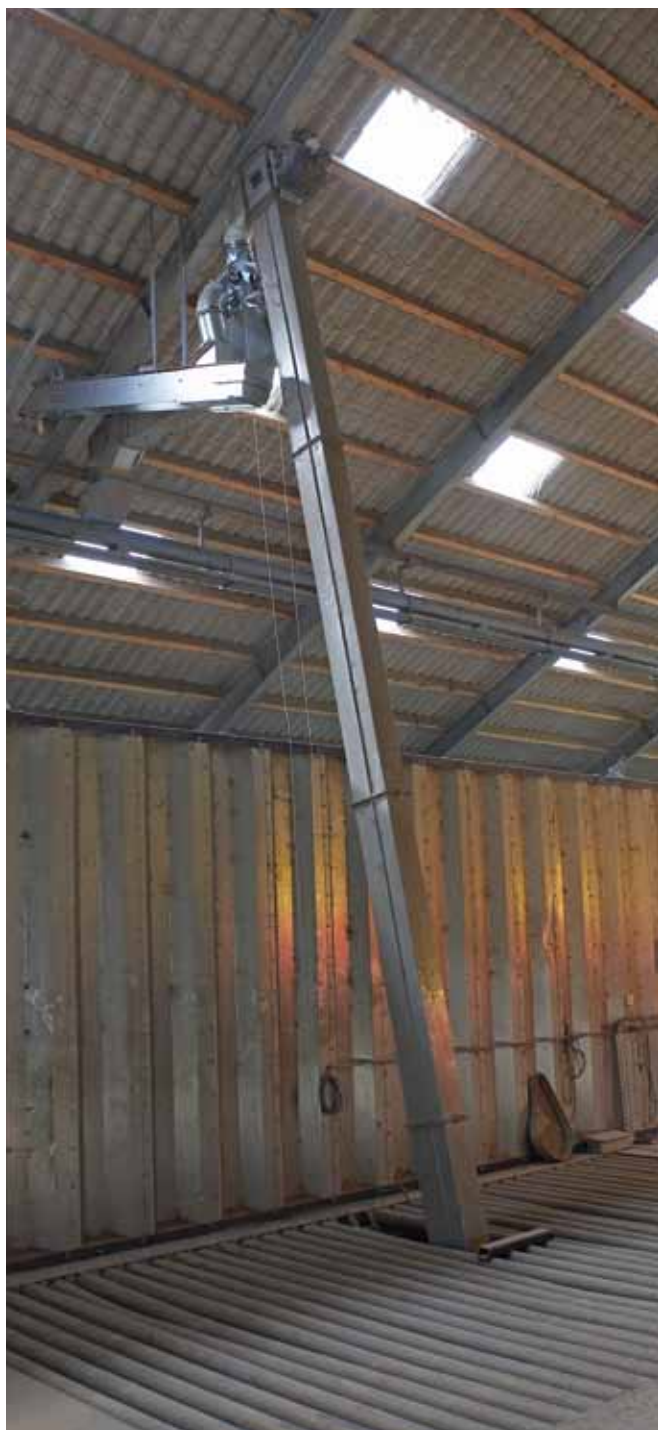
Chain elevator with a capacity of 20 t/h and 40 t/h
