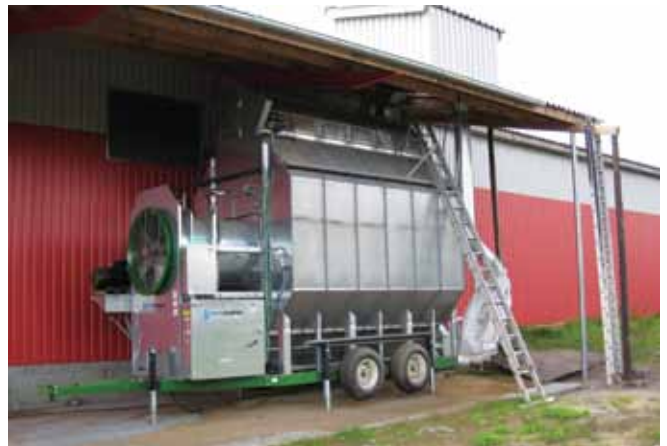
DC 12 mobile dryer with axial fan
