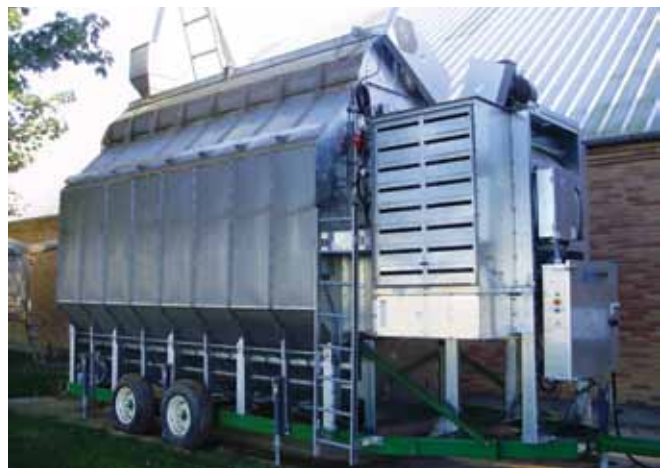
DCC163 mobile dryer with centrifugal fan
